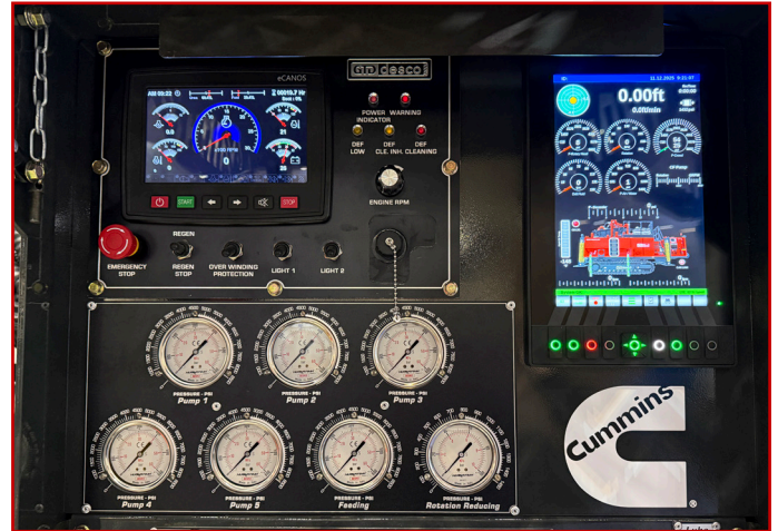
(Live data read-outs positioned above main drillers controls)
