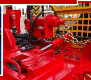
HYDRAULIC SLIDING ROD WRENCH
