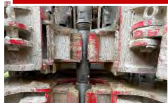
TRIPLE CLAMPS 1 ROTATING & 2 FIXED 12½" (320 mm) OPENING
