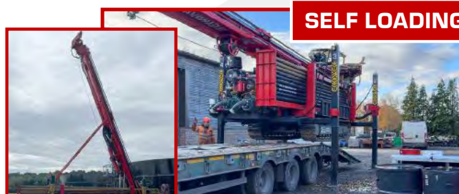
4 x HYDRAULIC LEGS TO LIFT & LEVEL THE RIG
