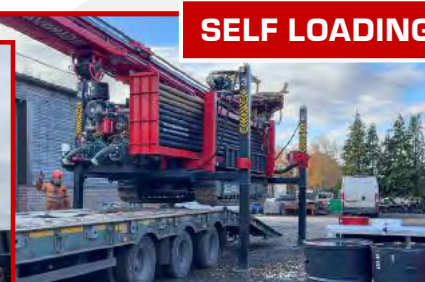
4 x HYDRAULIC LEGS TO LIFT & LEVEL THE RIG
