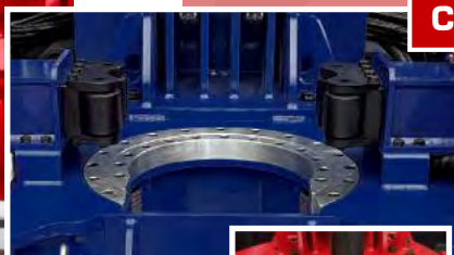
HYDRAULIC CENTRALIZING ROLLERS
