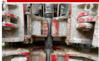
TRIPLE CLAMPS 1 ROTATING & 2 FIXED 12½" (320 mm) OPENING
