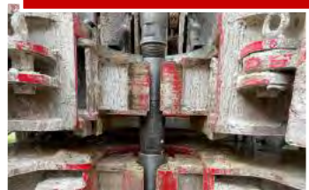
TRIPLE CLAMPS 1 ROTATING & 2 FIXED 12½" (320 mm) OPENING
