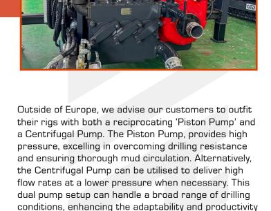
In Europe, it is more typical to have a dual pump setup comprising of a Single Stage Centrifugal pump and a Multi Stage Centrifugal pump. The Single Stage pump delivers a high flow rate at lower pressure, or if necessary, the Multi Stage pump is invaluable in scenarios which require higher pressures.
